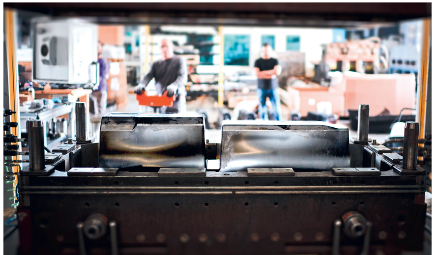
Large-area components, like the battery cover shown, can be produced very well using direct long fiber compression molding. Optimized materials such as PA66 Mobius NPD 555 FR GF50 from Invista are ideal for the process involved. © Invista
